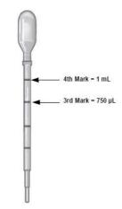
Figure 6. HIV-1 Qual Assay 1 mL Transfer Pipette
